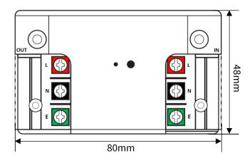
It is normal for any dimmer to produce small amounts of audible noise or buzzing. The noise may vary according to the dimmer setting. Incompatible load types: Ceiling sweep fans, exhaust fans and non-dimmable light sources
